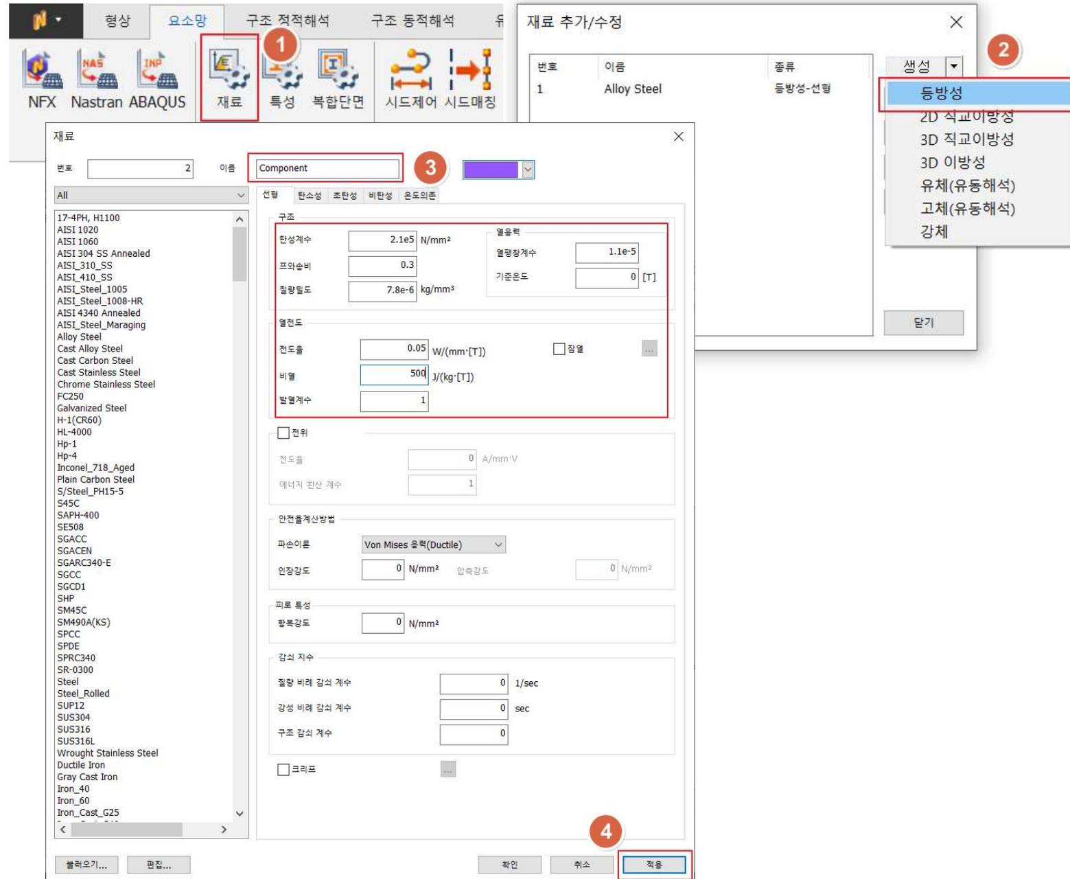
The screenshot shows the Midas NFX software interface. The '재료' (Material) button is highlighted with a red box and a '1' callout. The '생성' (Generate) dropdown menu is open, showing '등방성' (Isotropic) selected with a red box and a '2' callout. The '재료 추가/수정' (Material Add/Edit) dialog box is open, showing the 'Component' material name and a '3' callout. The '적용' (Apply) button is highlighted with a red box and a '4' callout.
